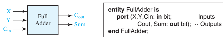
FIGURE 10-10 Entity Declaration for a Full Adder Module
